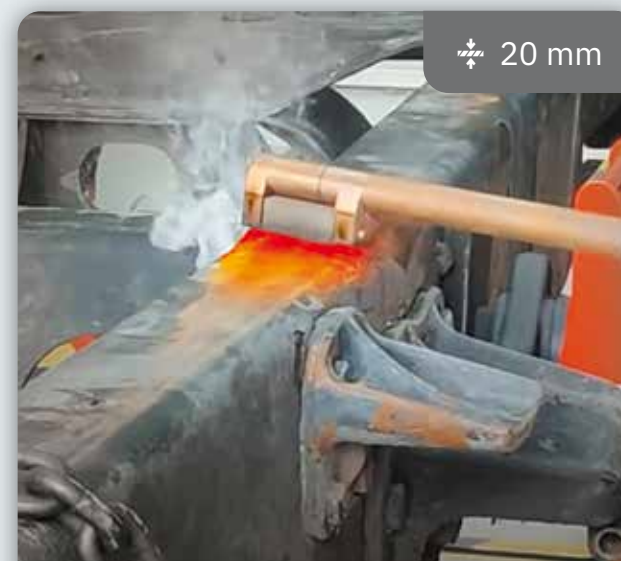
TRUCK CHASSIS STRAIGHTENING - REDRESSAGE CHASSIS DE CAMION Large L90 Powerduction 220LG
