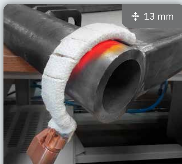
BUCKET PIN EXTRACTION - EXTRACTION DES AXES DE GODETS Large L180/D120H Powerduction 220LG
