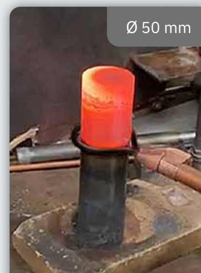
STEEL BAR FORGING - FORGEAGE BARRE ACIER Large L180/D60 Powerduction 220 LG
