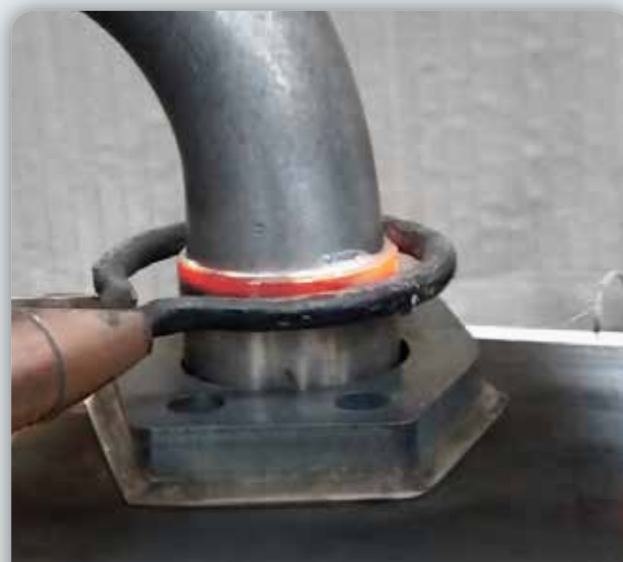
BRAZING STEEL ELBOW - BRASAGE COUDE ACIER Large L180/D120 Powerduction 160 LG
