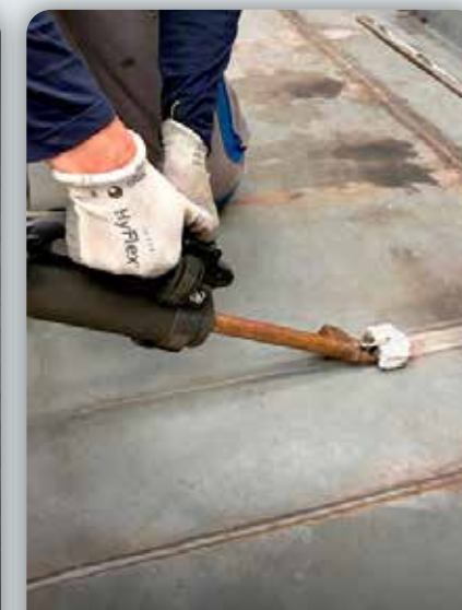
SHIPYARD - HEAT SHRINKING - CONSTRUCTION NAVALE - CHAQUE DE RETRAIT Large L20/B4 Powerduction 220LG
