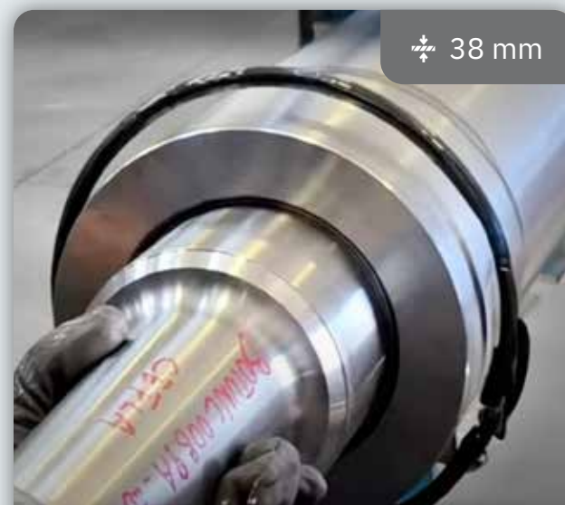
STEEL TUBE SHRINK-FITTING - FRETAGE DE TUBE ACIER Large L180/D300(on demand) Powerduction 220LG
