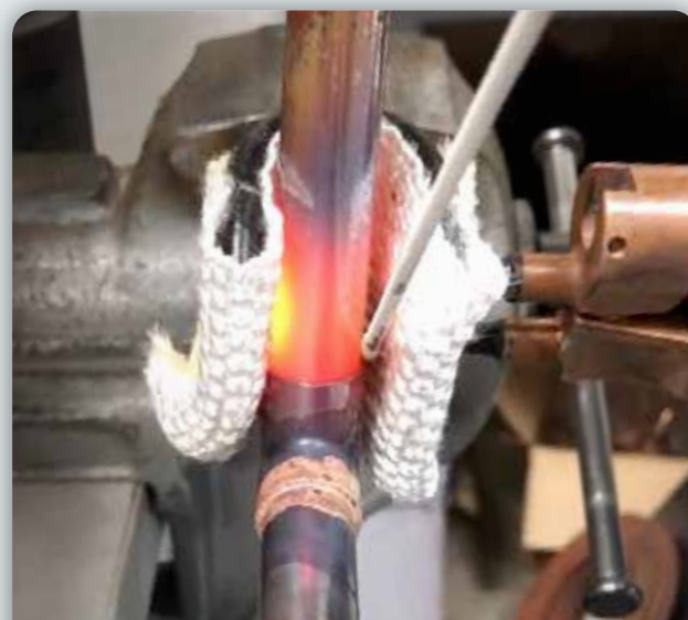
BRAZING COPPER PIPE - BRASAGE TUYAU CUIVRE Large L90 BRAZ 16 Powerduction 110 LG
