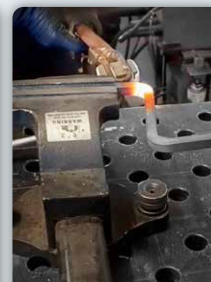
STEEL BAR BENDING - CINTRAGE BARRE ACIER Large L20/B4 Powerduction 110 LG
